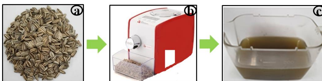
Figure 2.2. Fresh oil extraction process. (a) Sunflower seeds; (b). Cold press machine oil extractor; (c). Container with crude sunflower oil.
